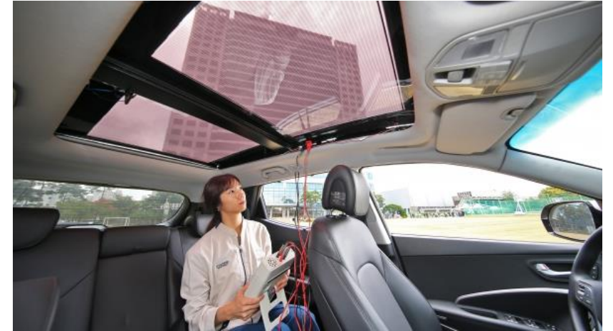
Hyundai (2018). Translucent solar roof engineering.
